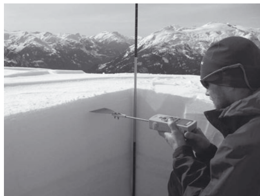
Fig. 4. Carrying out a blade hardness measurement with the blade oriented parallel to the stratigraphic layering.
