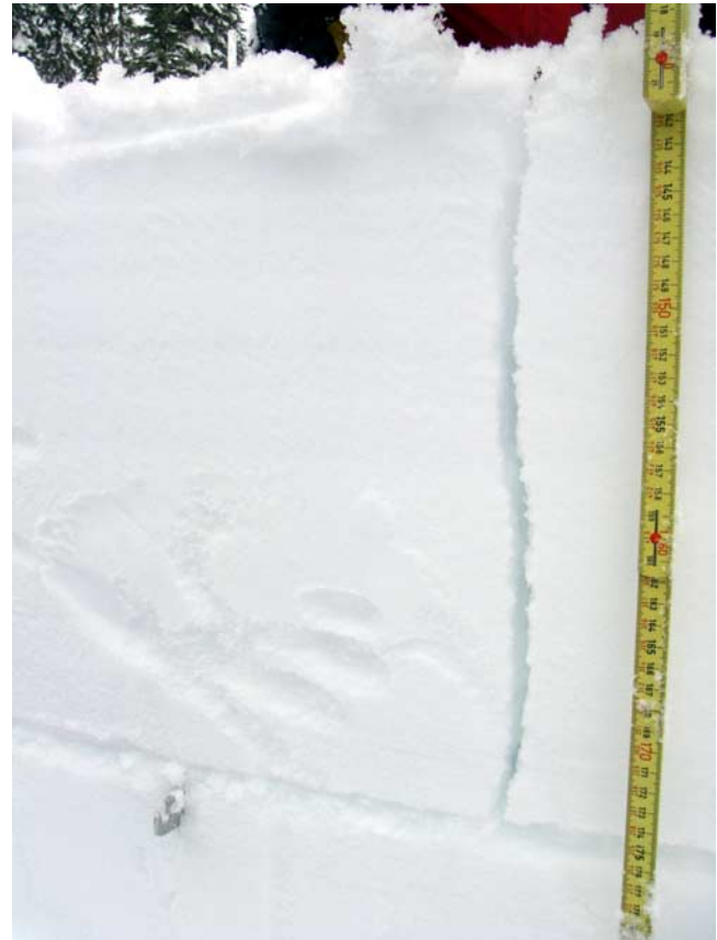
Figure 1b. Photo of fractures observed in field tests on horizontal terrain (slope angle 0^\circ ). The shear fracture initiated at the position where the saw is located by cutting through the weak layer from left to right. Tensile fracture through the slab occurred after the shear fracture propagated for about 20 cm. Photo courtesy of R. Burrows.
