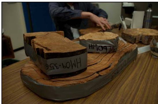
Wood samples, RA filling cracks with glue in background
