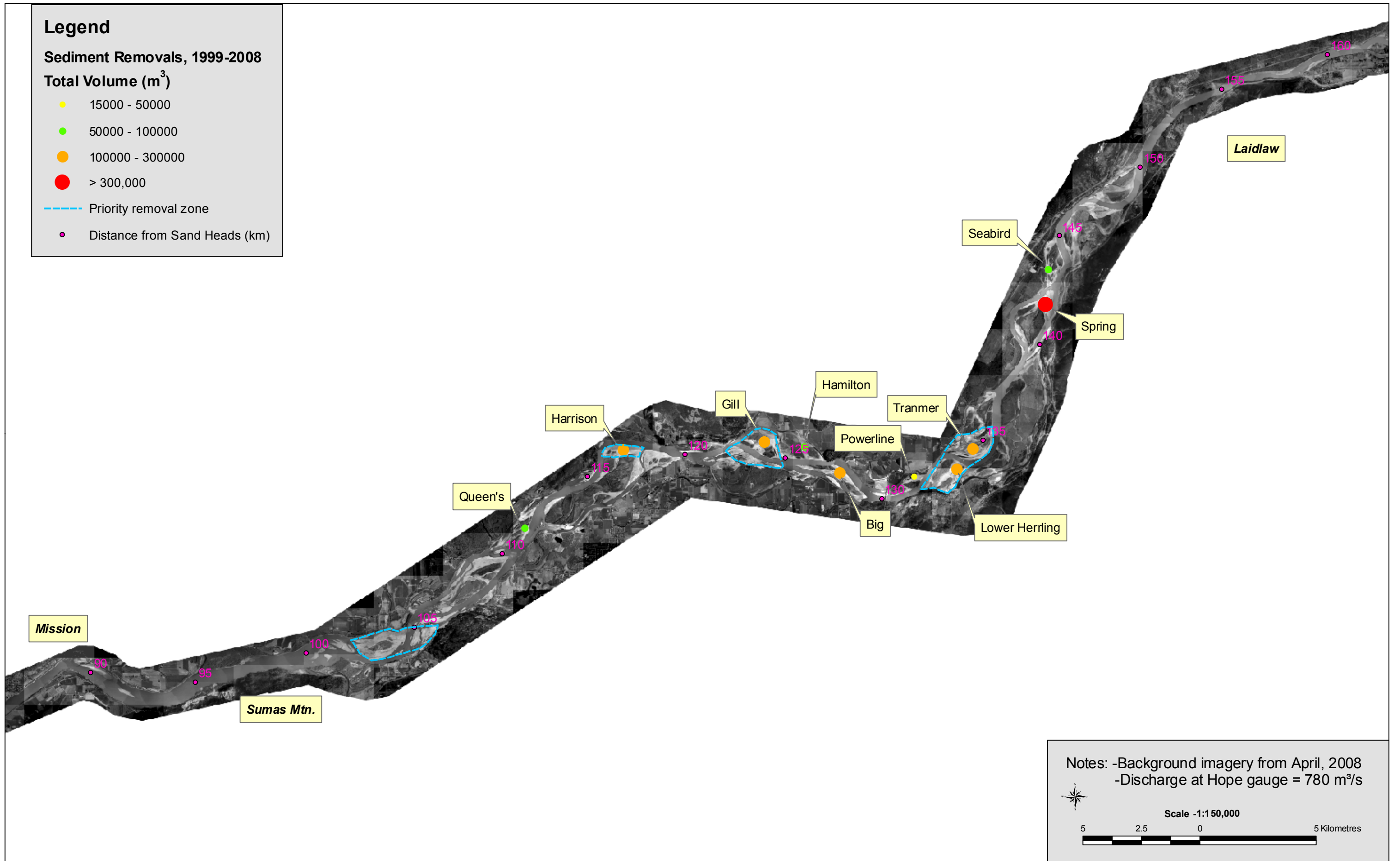
Figure 1: Location of sediment removals, 2000 - 2009 (modified from nhc, 2009; their Figure 2.1)
