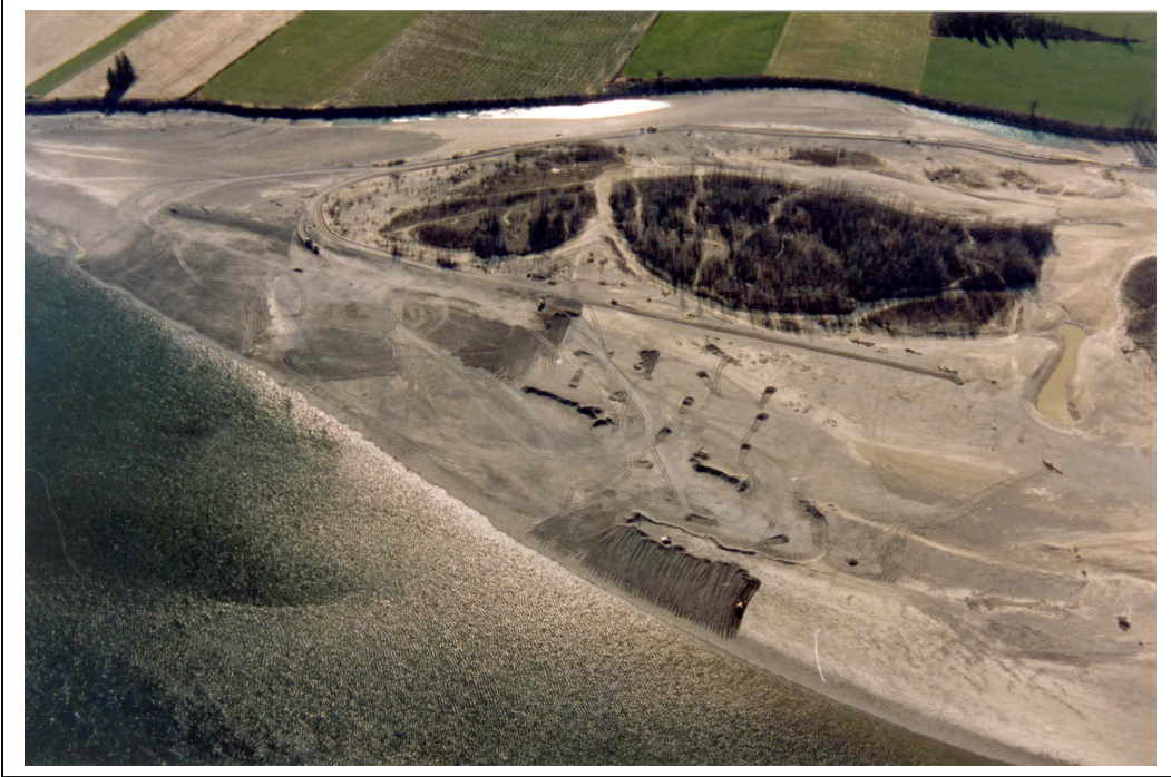
Bar scalping at Foster Bar. Photo taken March 2, 1995 (courtesy of Dr. V. Galay). Scalping took place in February/March 1995. Approximately 300,000 tonnes of gravel was removed.
