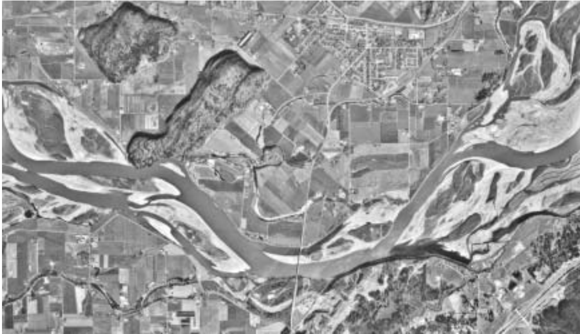
Figure 2-6. Characteristic wandering river morphology of the gravel reach, Fraser River (at Agassiz). Flow is from right to left (photo taken March 27, 1999; discharge: 700 \text{ m}^3 \text{ s}^{-1} ).
