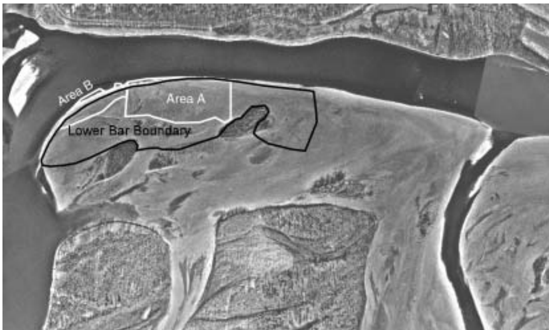
Figure 7-6. The three boundaries within which calculations of volumetric change between survey dates were made. Photograph taken March 7, 2001.
