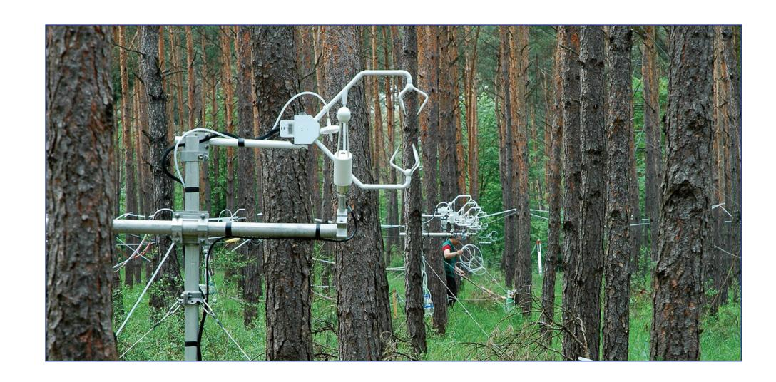
The field experiment HX06 was designed to quantify rarely measured spatial statistics in canopy turbulence. In particular, two-point correlations of velocity fluctuations, temperature, water vapor, and carbon dioxide were experimentally determined in the trunk space of a forest. Further, convection velocity was estimated for selected runs.
