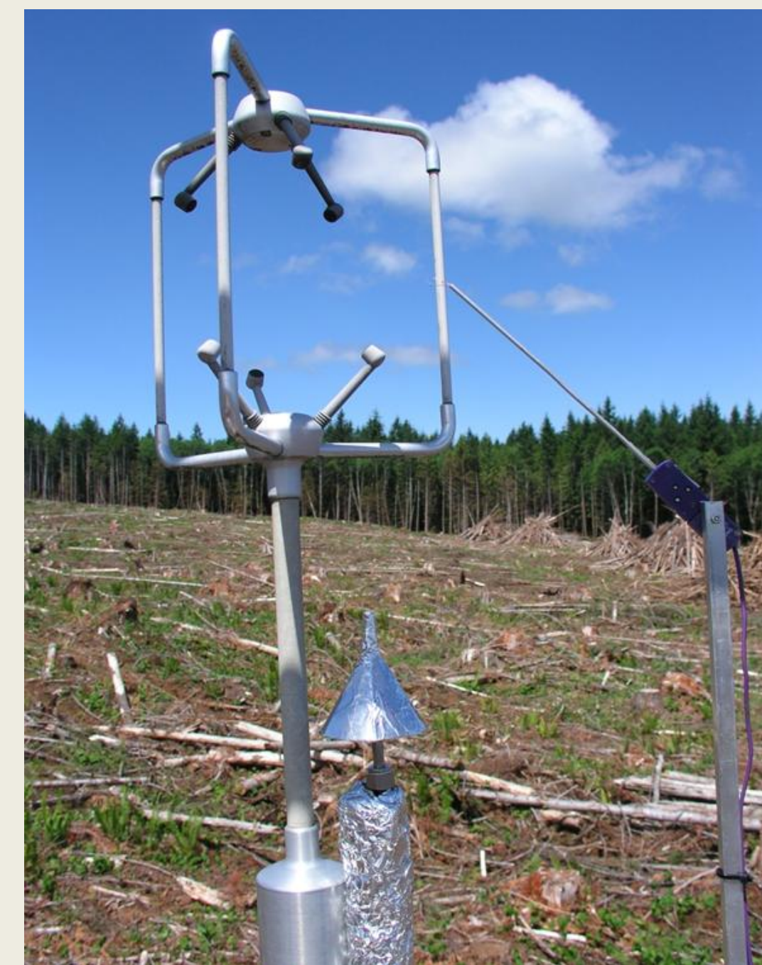
Fig. 2 Closed-path eddy covariance system at a height of 4.5 m above the ground. Measurements are taken at a frequency of 20 Hz and calibrations are done daily.
