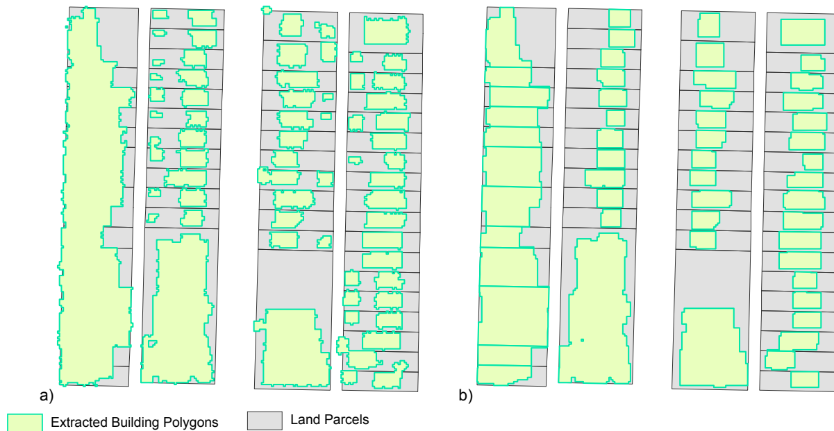
Figure 2.2.1: Results of the extraction techniques to derive primary buildings, trees, and ground vegetation using LiDAR data and Quickbird satellite imagery.
