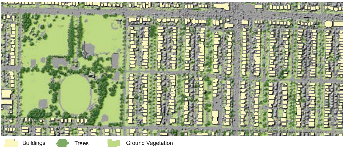
Figure 2.2.2: A city block in study area that displays a) resulting building polygons from the LiDAR extraction technique, and b) resulting building polygons after post-processing to simplify polygon shapes, remove secondary structures, and separate buildings by land parcel boundaries.
