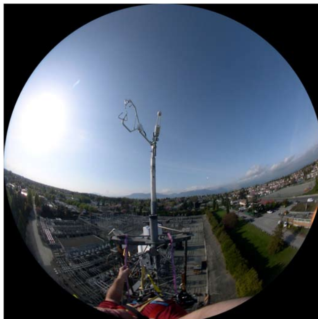
Figure 2.7.3: Photo of the EC instrumentation on top of the carbon flux tower taken with a fisheye lens. The sonic anemometer is on the left, the gas analyzer on the right. Both instruments are mounted 28.8 m above the local surface (Photo by R. Ketler, UBC).
