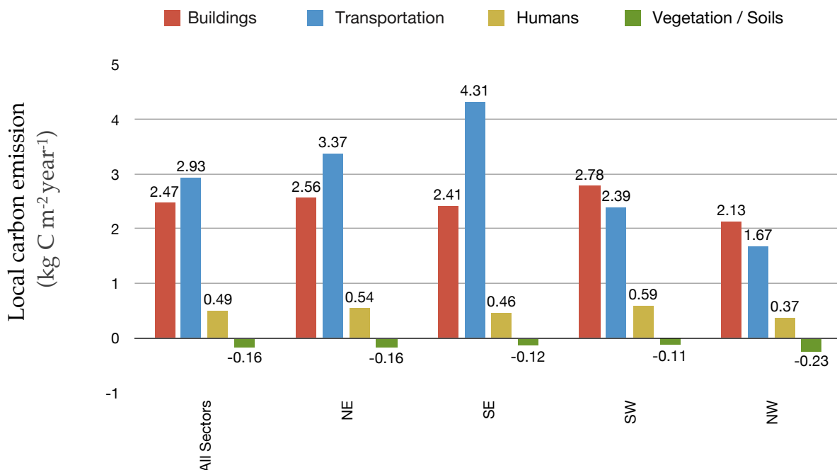
Figure 3.5.1: Comparison of the different emission components in the whole study area and for the different sectors. Vegetation shows the net-effect incorporating both, uptake and emissions.
